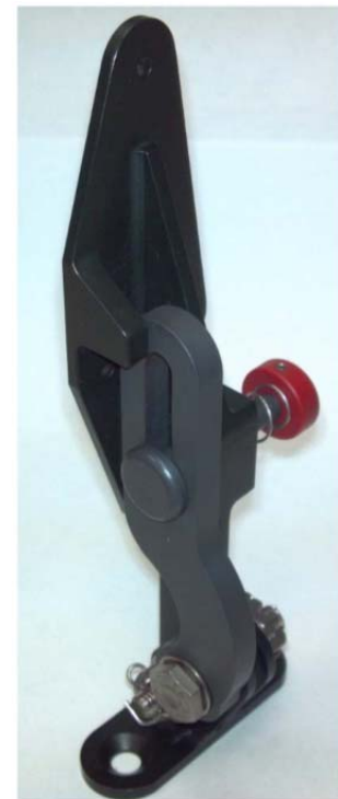
Figure 3 Hinge, Locking Assembly (Baggage Bay Door Locked Open)
